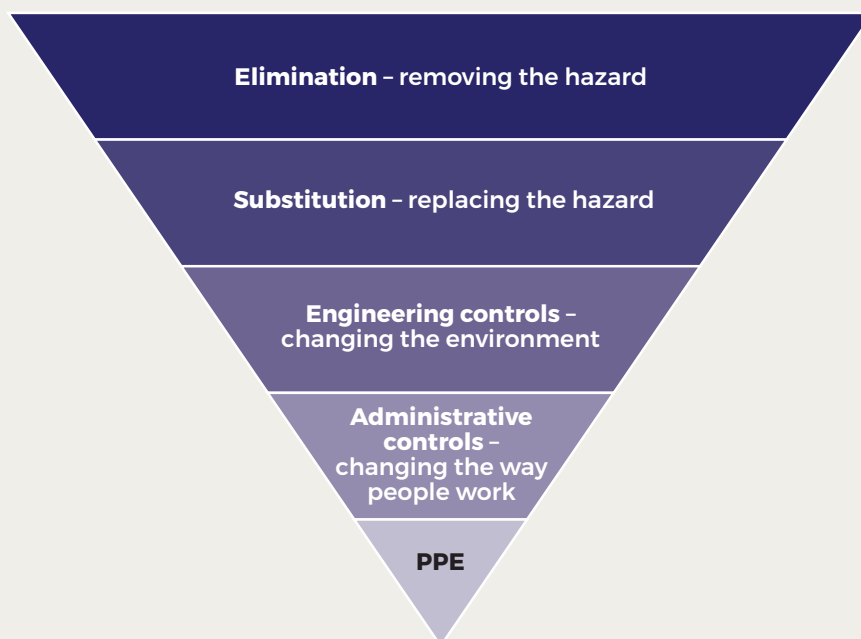
Figure 1.2. Infection prevention and control: Hierarchy of controls to be applied in order of priority 22
